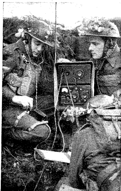
BATTALION SIGNALLERS AT WORK. This photograph, taken during recent exercises in Northern Ireland, shows a transmitting key strapped to the operator's thigh. It gives a tolerably good operating position and a more stable "platform" than might otherwise be obtainable in the field.
